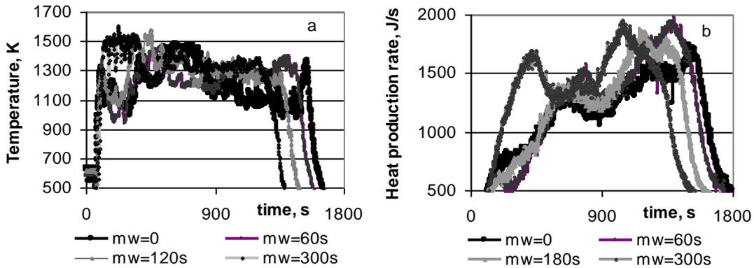
Figure 4: Effect of the microwave pre-treatment duration on the time-dependent variations of temperature (a) and heat production rates (b) at different stages of thermo-chemical conversion.
