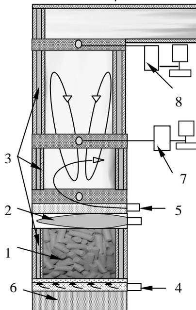
Figure 1: Principal schematic drawing of the experimental set-up: 1 - gasifier, charged with biomass pellets; 2 - additional heat energy supply from propane flame flow; 3 - water-cooled sections of the gasifier and the combustor; 4 - primary air supply; 5 - secondary air supply; 6 - ash collection vessel; 7 - flame temperature online measurements; 8 - online measurements of the combustion efficiency and composition of the products.
