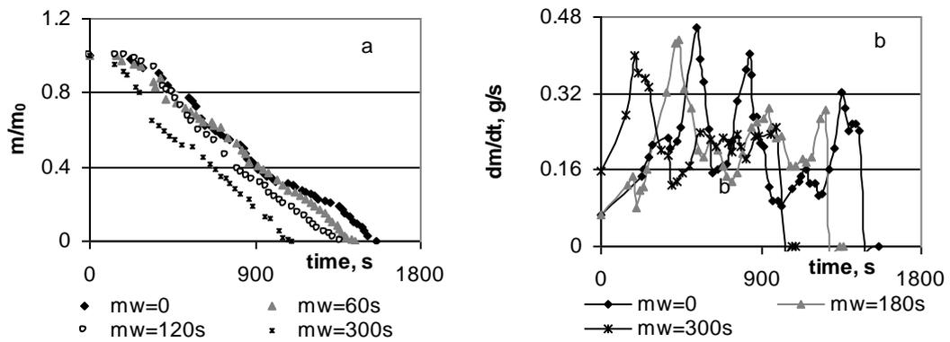
Figure 2: Effect of the microwave pre-treatment duration on the relative mass loss (a) and mass loss rate variations (b) of pre-treated samples at different stages of thermo-chemical conversion.
