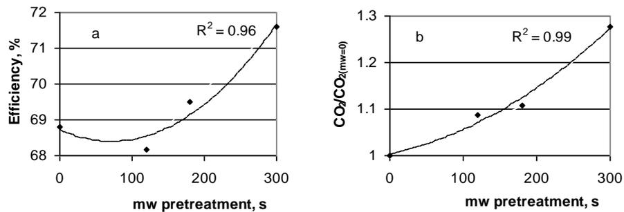
Figure 5: Effect of the microwave pre-treatment duration on the variations of combustion efficiency (a) and  $\text{CO}_2$  volume fraction (b).
