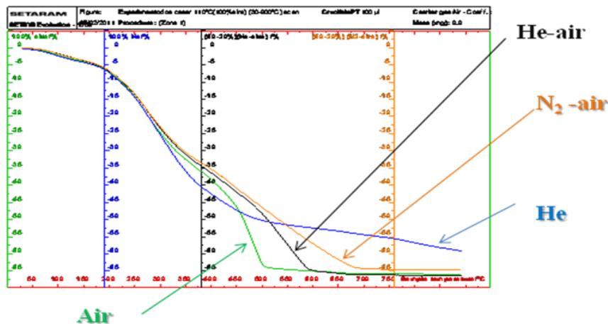
Figure 1. Mass loss profiles for dry sewage sludge of Casar de Periedo in different atmospheres.
