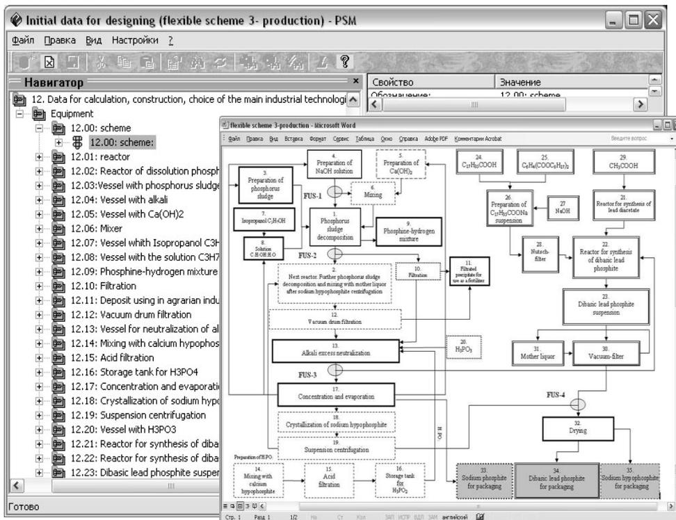
Figure 2. Element of the CALS-project "Initial data for design": the flexible three-product scheme for the phosphoric sludge processing
