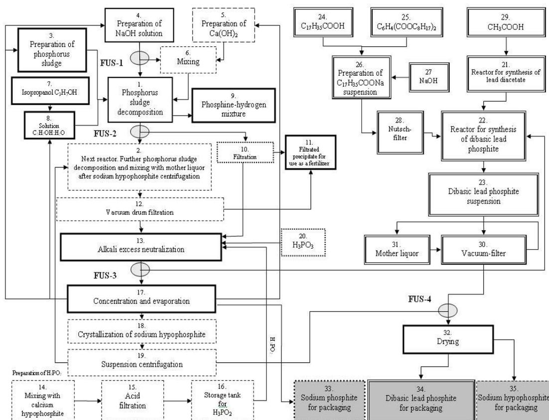
Figure 1. The flexible technology for production of sodium phosphite, sodium hypophosphite and dibasic lead phosphite
