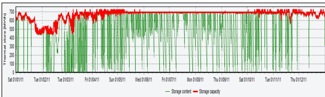
Figure 4: Charging and recharging of accumulator tank
