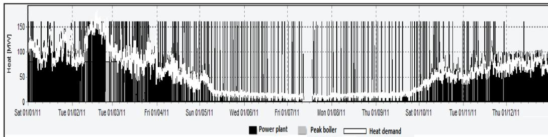
Figure 2: Heat supply by the Balti Power plant and peak boiler
