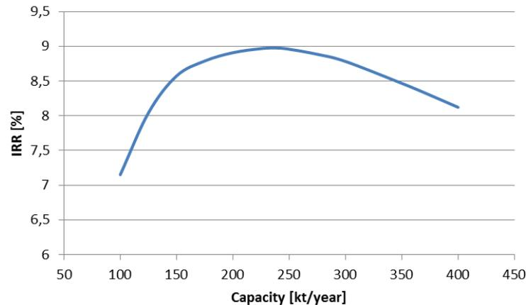
Figure 4: Sensitivity of IRR to waste treatment capacity
