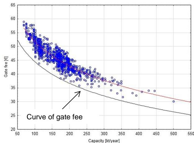
Figure 3: The gate fee curve used in the model
