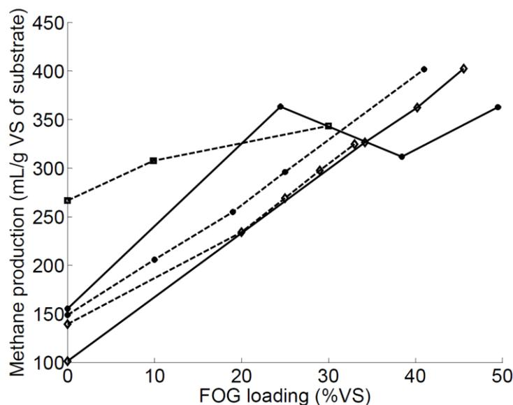
Figure 2: Methane production in co-digestion of sludge and FOG: the first batch run (●-) and the second run (◇-) are compared with the results of batch-tests done by Kabouris et al. (2008) with normal seed sludge (●-) and acclimatized seed sludge (◇-) and Davidsson et al. (2008). All results volumes are corrected in reference to the inoculum and are normalized to 25°C. The methane fraction is about 65 %.
