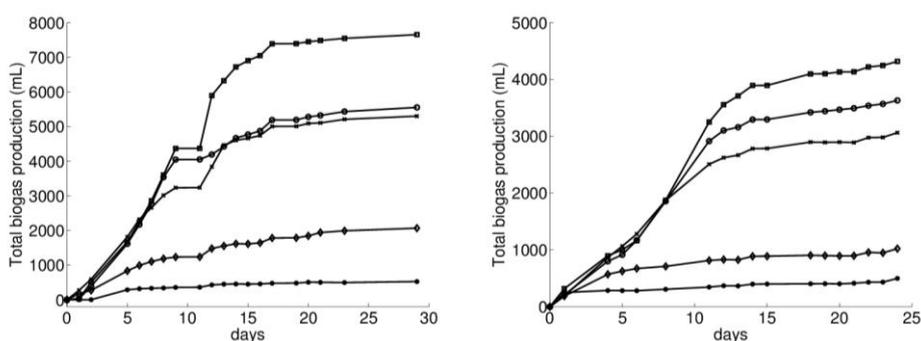
Figure 1: Total biogas production in time. Left: run 1 for the seed (-●-) and sludge-oil mixtures with an FOG fraction of 0% VS (-◆-), 24.5 % VS (-x-), 38.4 % VS (-o-) and 49.5 % VS (-■-). Right: run 2 for the seed (-●-) and sludge-oil mixture with an FOG fraction of 0 % VS (-◆-), 34.2 % VS (-x-), 40.2 % VS (-o-) and 45.5 % VS (-■-).
