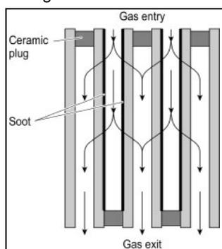
Figure 1: Wall Flow Filter (DPF)
