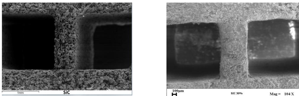
Figure 3: SEM images of the frontal channels of an uncatalysed SiC DPF (on the left) and a catalysed DPF with 30 %wt of  $\text{CuFe}_2\text{O}_4$  (on the right)
