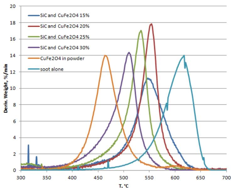
Figure 5: TG test performed on soot alone, soot and  $\text{CuFe}_2\text{O}_4$ , soot and SiC WFF with 15 %wt, 20 %wt, 25 %wt and 30 %wt of  $\text{CuFe}_2\text{O}_4$
