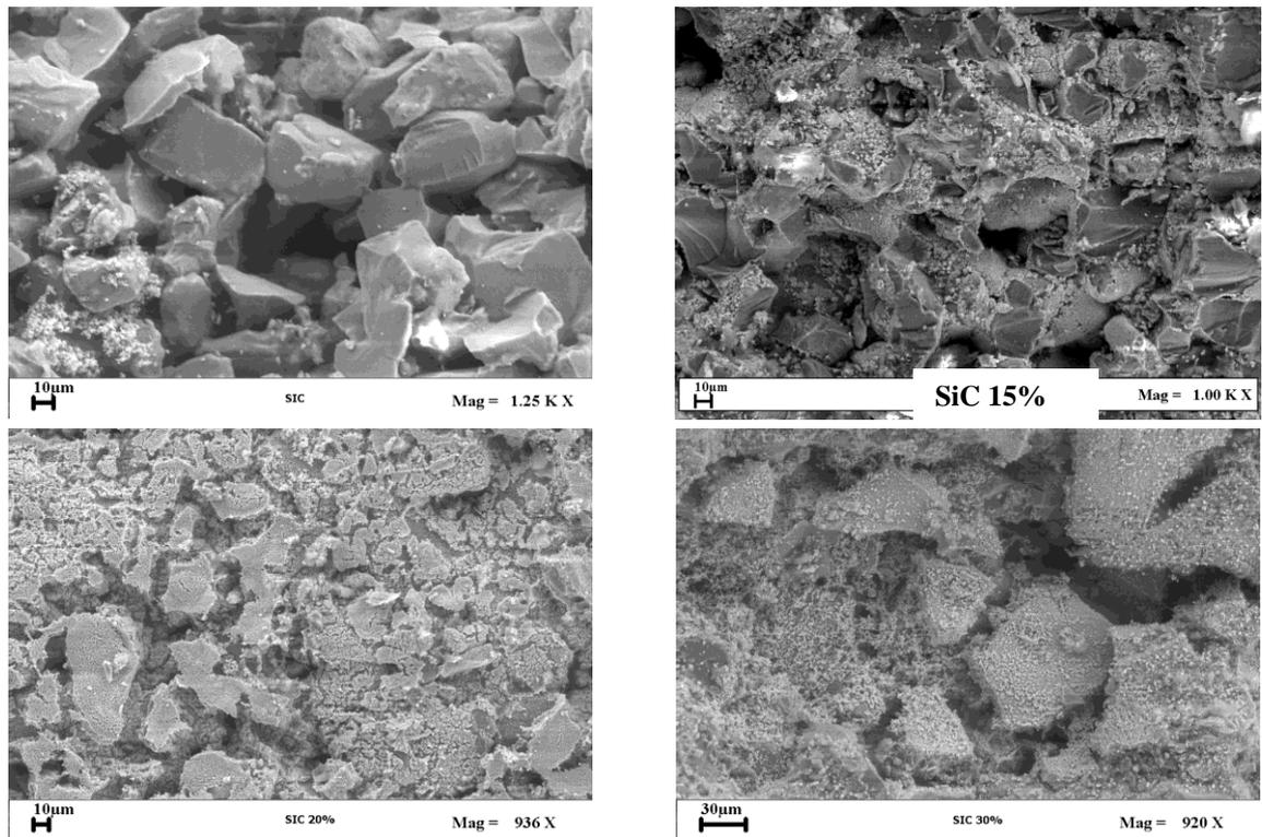
Figure 4: SEM images of the uncatyalsed DPF and of the catalysed DPF with 15%, 20% and 30%wt of  $\text{CuFe}_2\text{O}_4$
