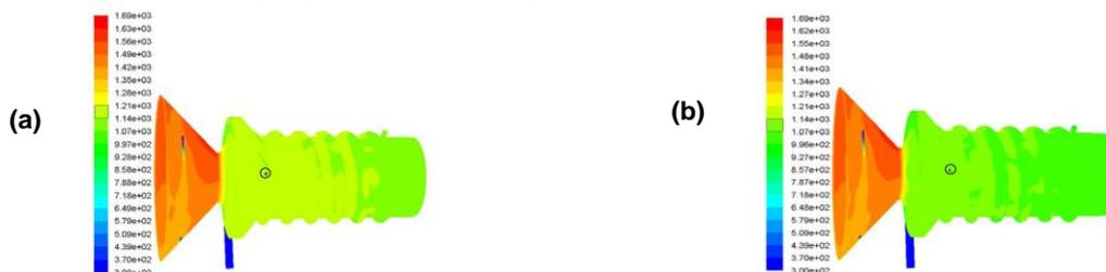
Figure 2: (a) contours of static temperature of reactor walls for  $m_p = 0.2$  g/min, (b) contours of static temperature of reactor walls for  $m_p = 0.6$  g/min
