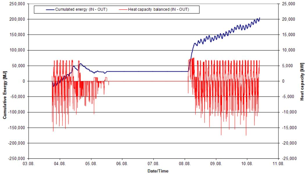
Figure 1: Evaluation of ingoing and outgoing energy and the cumulated energy in the energy storage evaluated (96 m<sup>3</sup>)
