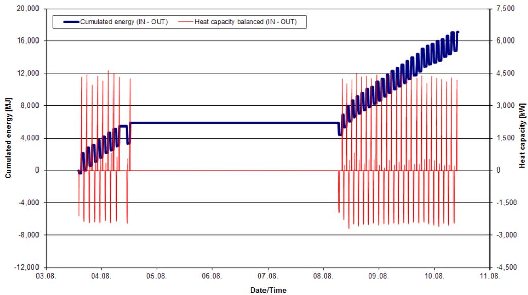
Figure 2: Evaluation of ingoing and outgoing energy and the cumulated energy in the hot water storage evaluated (220 m<sup>3</sup>)
