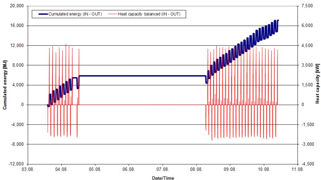
*Figure 2: Evaluation of ingoing and outgoing energy and the cumulated energy in the hot water storage evaluated (220 m<sup>3</sup>)*
