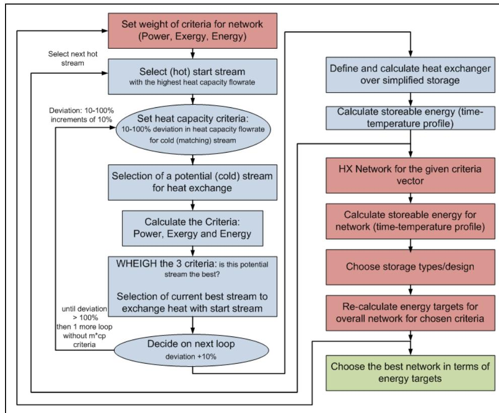
Figure 3: Structure of the algorithm of the SOCO tool
