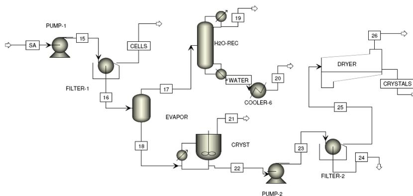
Figure 2: Flowsheet of the downstream process of succinic acid after the fermentation procedure (Vlysidis et al., 2011a).
