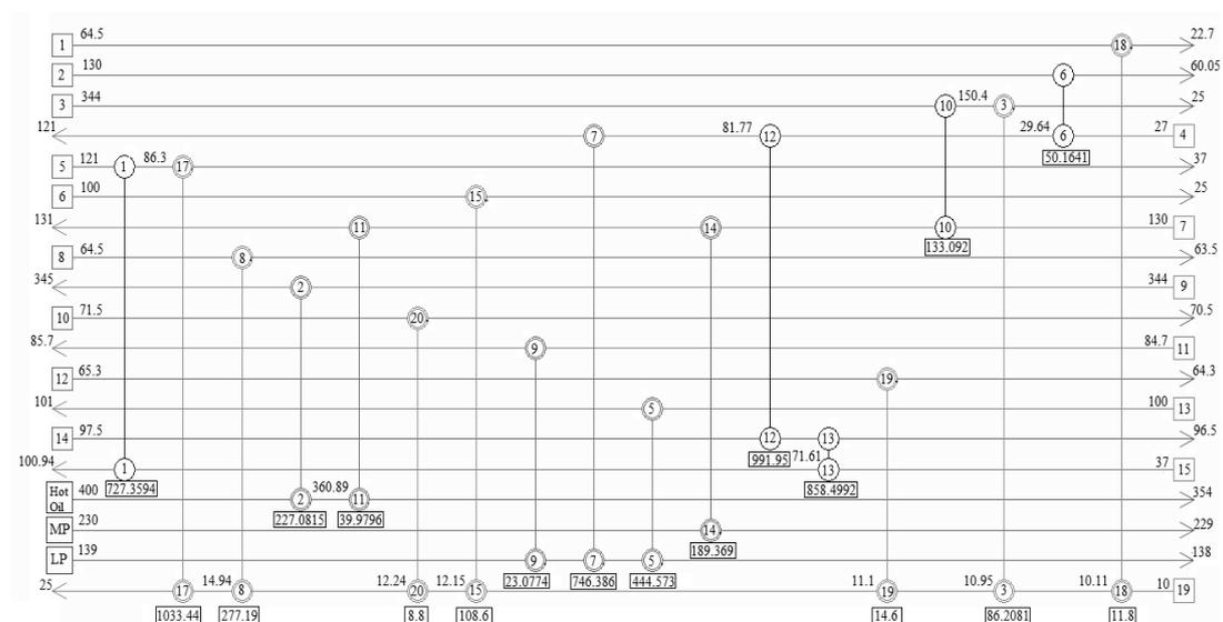
Figure 5: Final HEN design for the biodiesel succinic acid biorefinery
