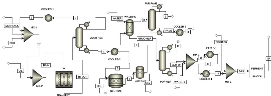
Figure 1: Flowsheet of integrated biorefinery for biodiesel production from vegetable oils and production of succinate through fermentation from crude glycerol (Binns et al., 2011).
