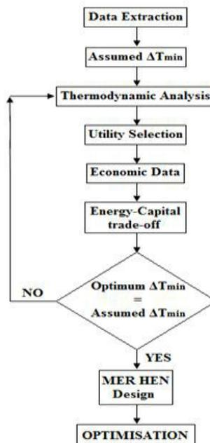
Figure 3: Methodology procedure for designing and optimising HENs
