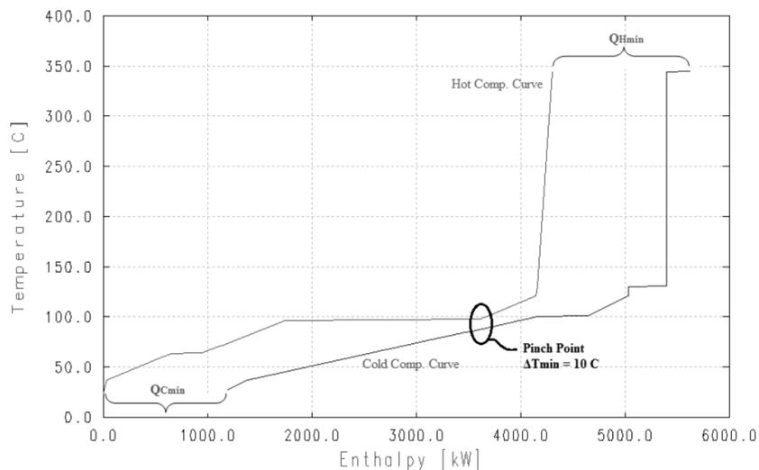
Figure 4: Composite curves of the overall biorefinery
