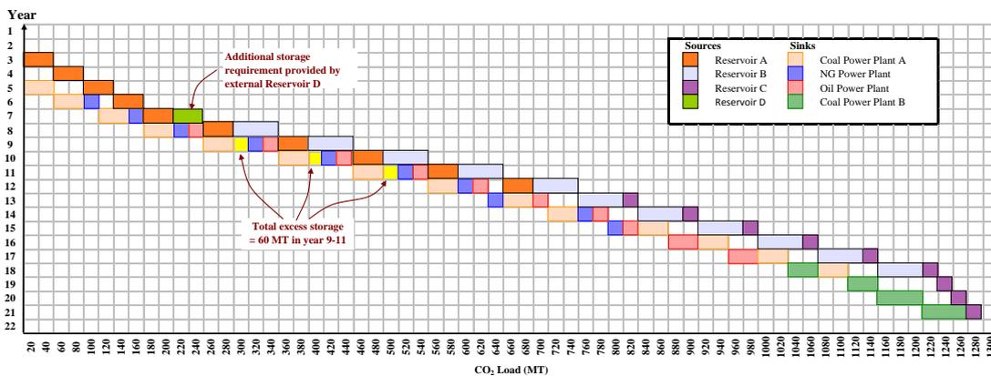
Figure 5: Detailed CSCC for matching of CO<sub>2</sub> sources with storage reservoir
