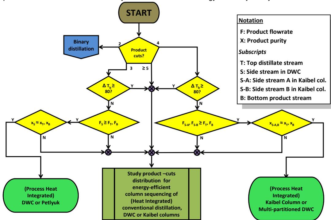
Figure 1. Main selection scheme of energy efficient distillation technologies
