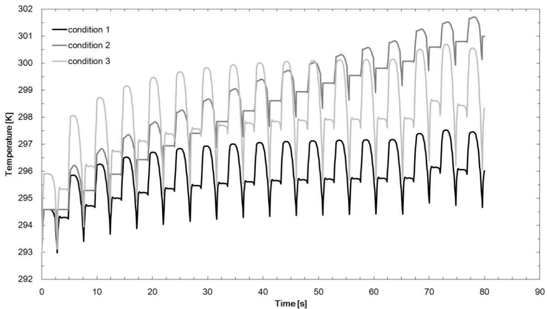
Figure 4: comparison of time evolution of particle bed hot end with reference (condition 1), larger bed length (condition 2), and large magnetic flux density (condition 3)
