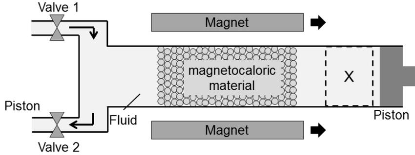
Figure 2: Configuration of magnetic heat circulator using packed bed with temperature gradient to obtain a quasi-counter flow heat exchange
