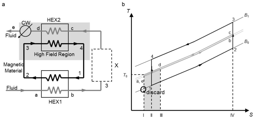
Figure 1: Schematic image of magnetic heat circulator a) process image b) cycle in terms of temperature-entropy diagram.  $T_0$  denotes the ambient temperature,  $B_0$  and  $B_1$  denotes the initial and high field region magnetic flux density respectively
