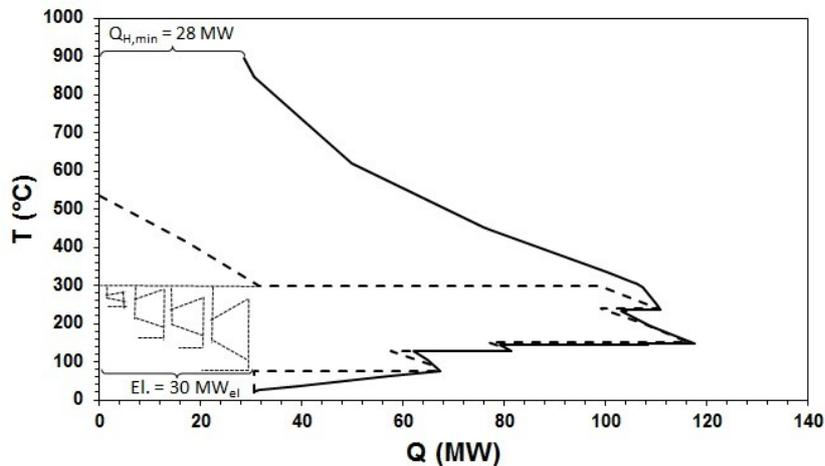
Figure 3: Background/foreground analysis – Integration between the SNG process sized to substitute the site's natural gas usage and a back-pressure steam cycle sized to cover the SNG and host site steam requirements and achieve maximum cogeneration (Case 3)
