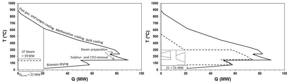
Figure 2: Background/foreground analysis - Integration between the SNG process sized to substitute the site's natural gas usage and the site's net steam demand (Case 1) (left), or a back-pressure steam cycle sized for maximum power generation from the available excess heat (Case 2) (right).
