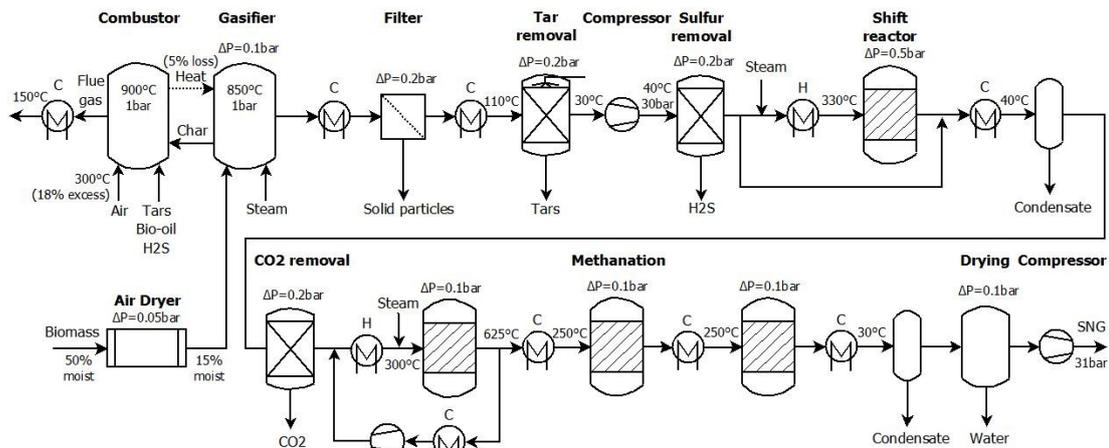
Figure 1: The SNG process configuration. Stream cooling requirements (heat sources) are noted with C, and streams requiring heating (heat sinks) are noted with H. The pressure drop for heating and cooling is assumed to be  $\Delta P/P = 2\%$ .
