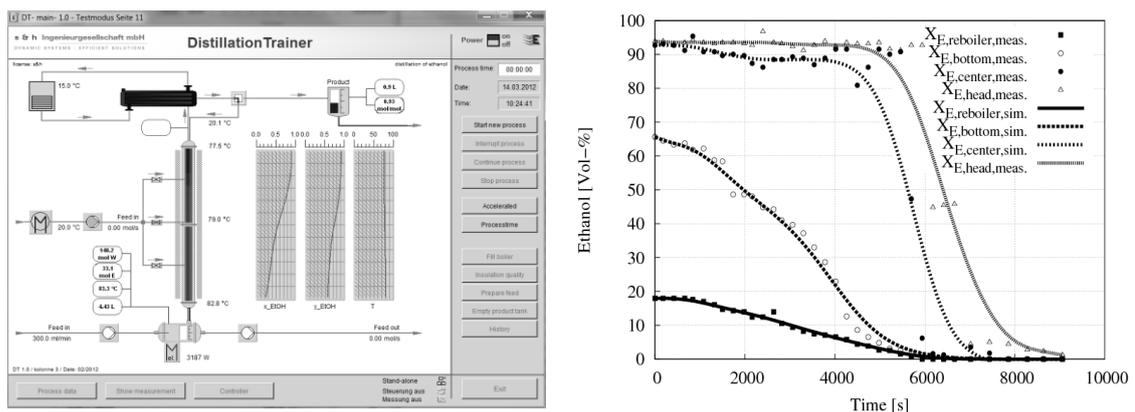
Figure 4: Left-side: Main GUI of the distillation simulator. In the middle-left position of the rectification column the connection to the bioethanol fermenter simulator is realised with an interface push-button. Right-side: Measured data (symbols) and simulated values (lines) of compositions in the head, centre, bottom of the column and the reboiler over time in a complete batch-distillation cycle of a water/ethanol mixture (right-side)
