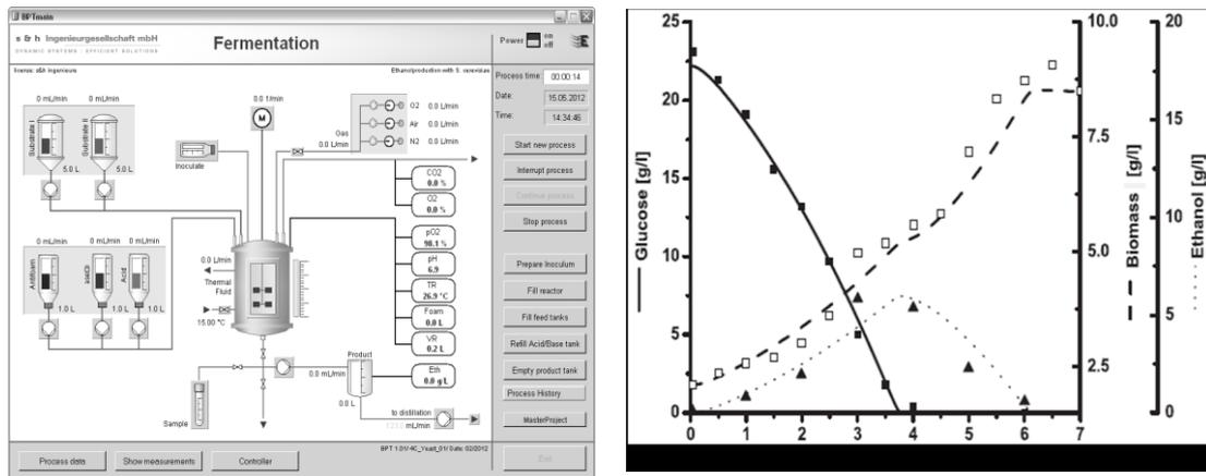
Figure 3: Left-side: Main GUI of the bioethanol fermentation simulator. In the bottom-right corner of the process control scheme the connection to the rectification simulator is realised with an interface push-button. Right-side: Measured (symbols) and simulated (lines) concentrations of glucose, ethanol and biomass (Hass, 2005).
