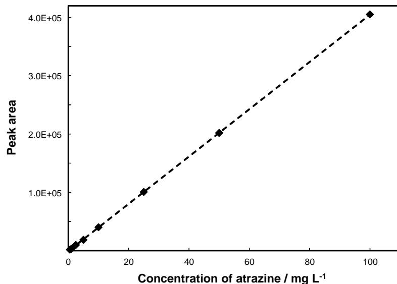
Figure 1: Chromatographic peak area as a function of atrazine concentration in acetone
