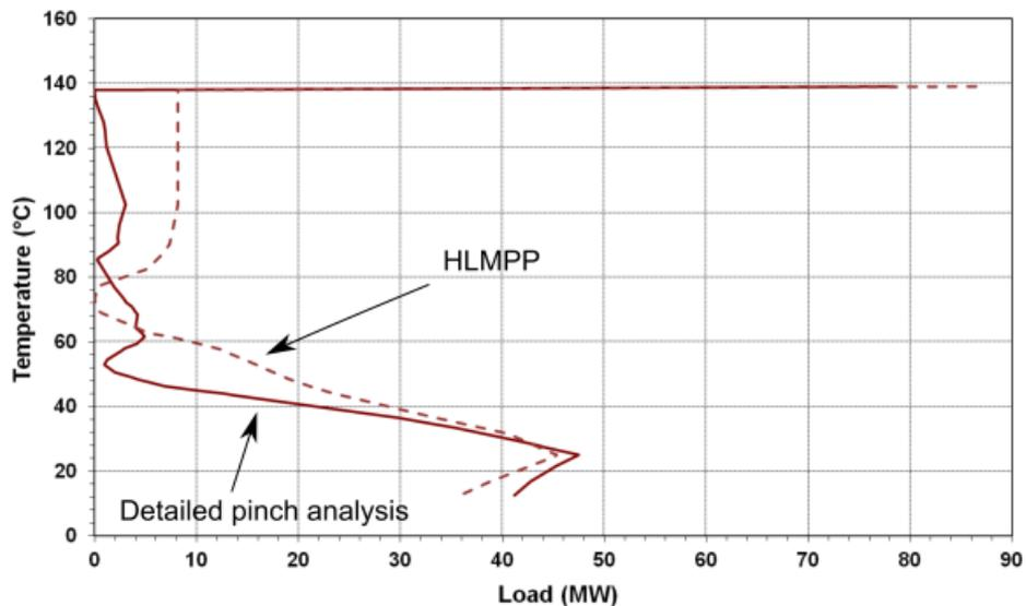
Figure 2: HLMPP GCC as dashed line and detailed pinch GCC as continuous line
