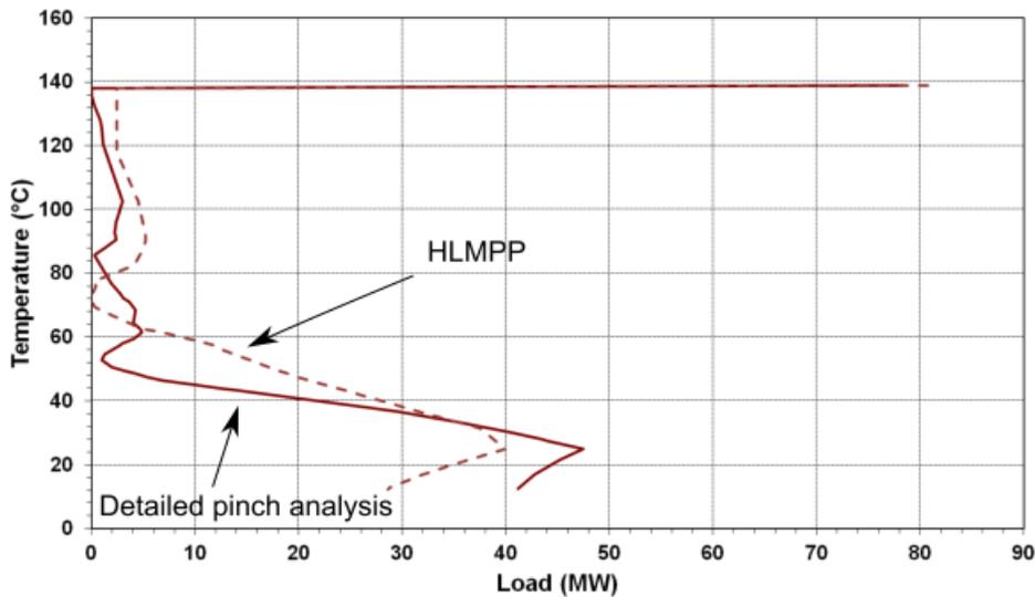
Figure 3: Detailed pinch GCC represented by a continuous line and HLMPP as dashed line, showing the influence of adding the dirty condensate stream in HLMPP (compare with Figure 2)
