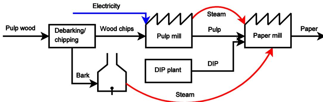
Figure 1: Principle layout of the TMP mill.
