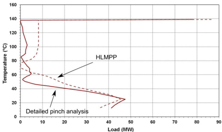
Figure 2: HLMPP GCC as dashed line and detailed pinch GCC as continuous line
