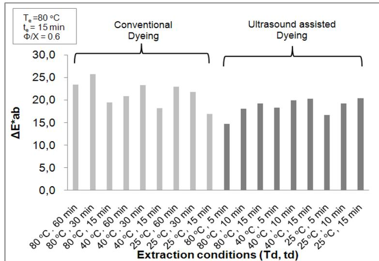
Figure 3: Effect of dyeing methods on total colour difference ( $\Delta E^*_{ab}$ ) in various conditions.
