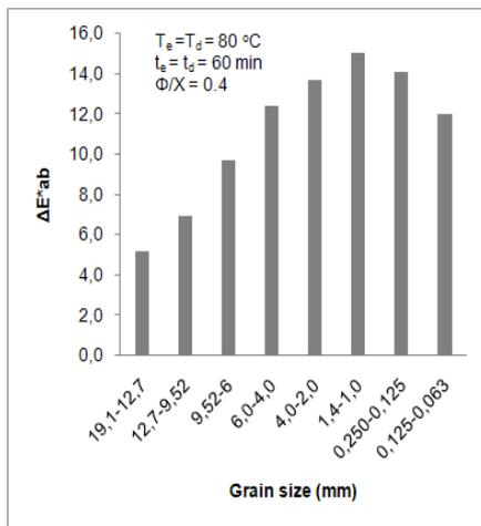
Figure 1: Grain size effect on total colour difference ( $\Delta E_{ab}^*$ ) at severe extraction and dyeing conditions.
