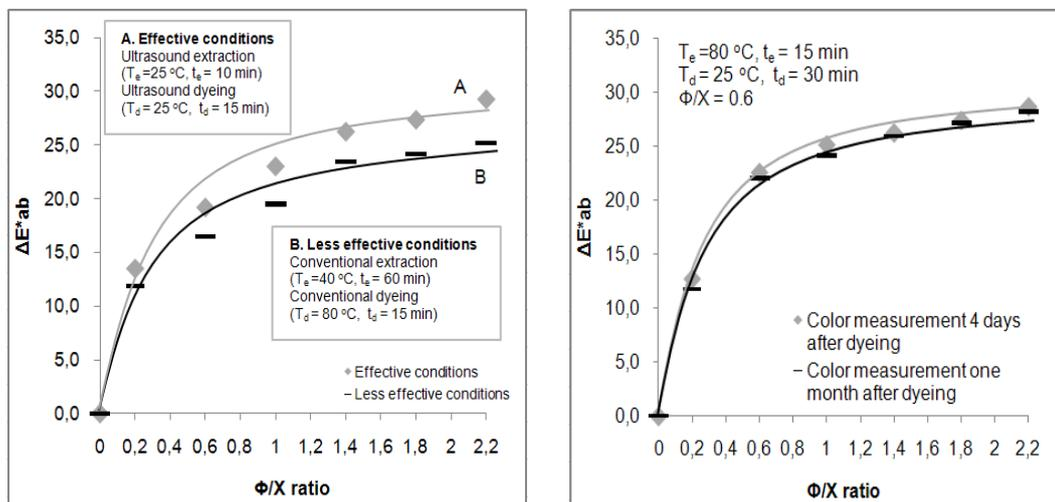
Figure 4:  $\Delta E^*_{ab}$  related with the  $\Phi/X$  ratio, comparison of effective and less effective conditions. Figure 5: Colour stability against ageing.
