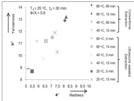
Figure 6: The impact of extraction methods on colour shade of dyed chemical pulp in various conditions.
