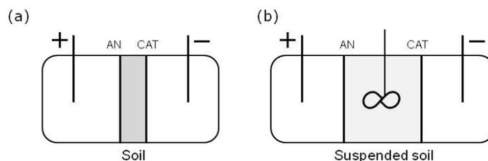
Figure 1: Schematics of the experimental cells (a) soil compacted and water saturated and (b) soil suspended in distilled water and stirred to keep in suspension during experiments. (AN = anion exchange membrane, CAT = cation exchange membrane)
