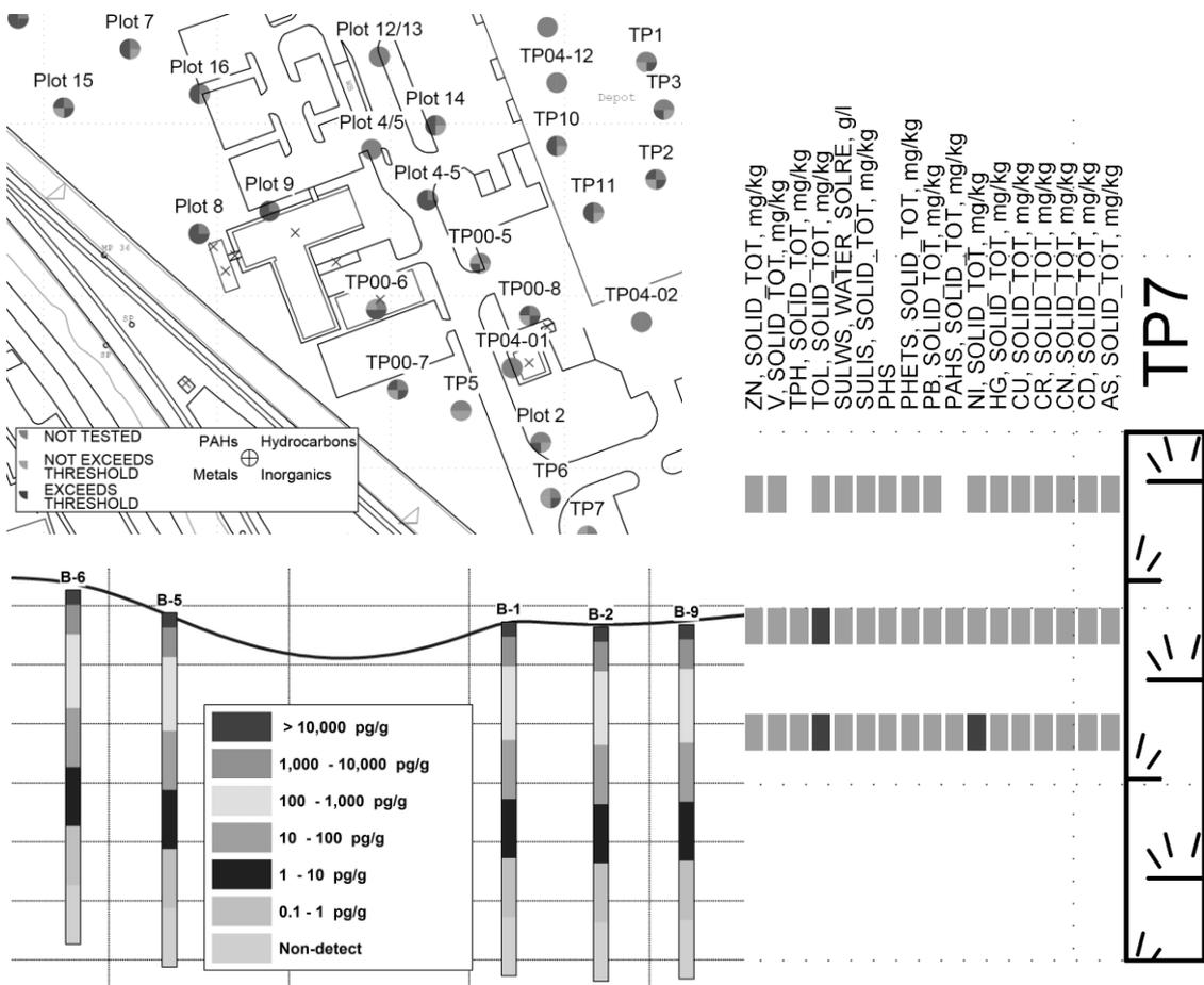
Figure 2: Example of various possible representations of same geoenvironmental data. The presence of determinants in figure, both on site map and profile is commonly shown in colour.
