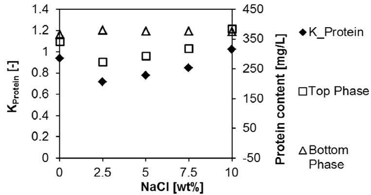
Figure 3: Protein partitioning coefficient and protein content of laccase from *Pleurotus sapidus* in an ATPS containing 12 wt.-% PEG 3000, 7 wt.-% phosphate and pH 7 with varying concentrations of sodium chloride.
