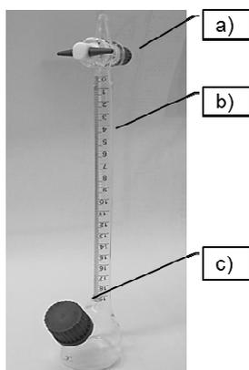
Figure 1: Extraction vessel consisting of burette valve a), burette b) and flask c).
