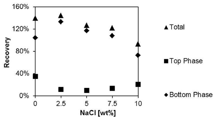
Figure 4: Activity recovery of laccase from *Pleurotus sapidus* in an ATPS containing 12 wt.-% PEG 3000, 7 wt.-% Phosphate and pH 7 with varying concentrations of sodium chloride.
