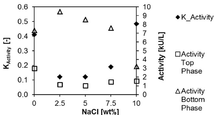
Figure 2: Activity partitioning coefficient and enzymatic activity of laccase from *Pleurotus sapidus* in an ATPS containing 12 wt.-% PEG 3000, 7 wt.-% phosphate and pH 7 with varying concentrations of sodium chloride
