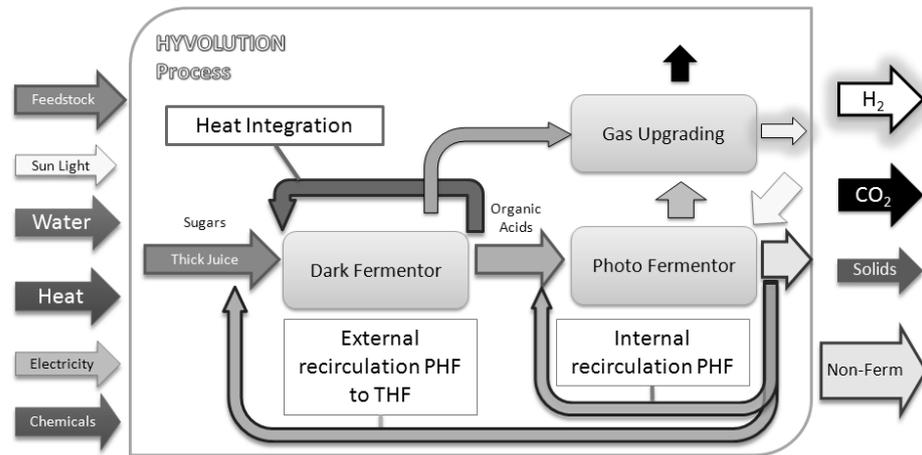
Figure 1: Scheme of HYVOLUTION process for Thick Juice.
