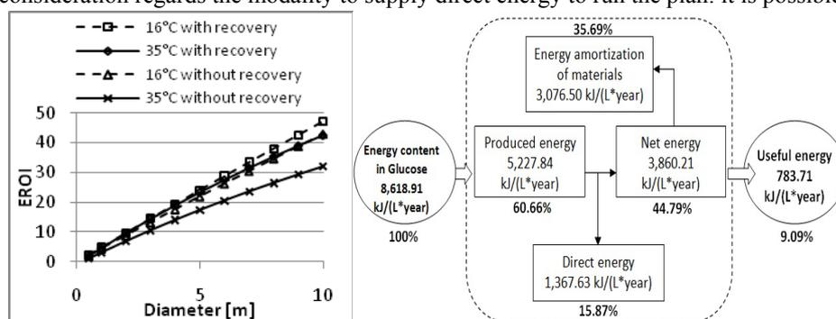
Figure 2: (Left) EROI for H<sub>2</sub> and CH<sub>4</sub> technology; (Right) Global energy balance for H<sub>2</sub> and CH<sub>4</sub> technology at T=35 °C with heat recovery, EPT=1, reactor diameter=4.
