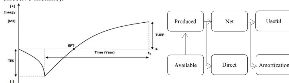
Figure 1: (Left) Global Net Energy Balance vs. Time; (Right) Energy flow-sheet of a generic process.
