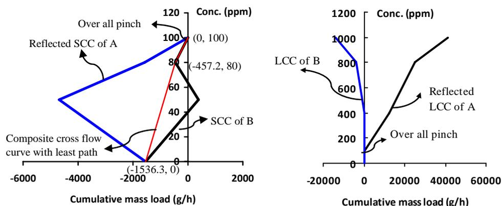
Figure 1: The reflected SCC of A and SCC of B as well as LCC of B and reflected LCC of A for the illustrative example.
