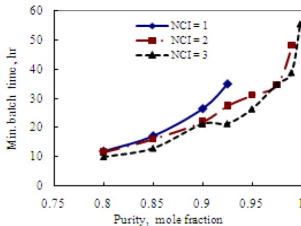
Fig.2. Total minimum operating time as a function of purity specification
