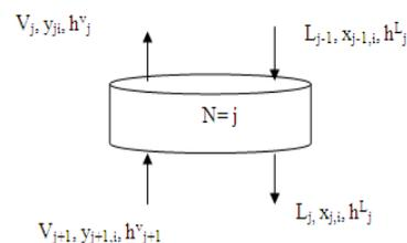
Fig. 1. Configuration and model equations for typical plate ( $N = j$ ).
