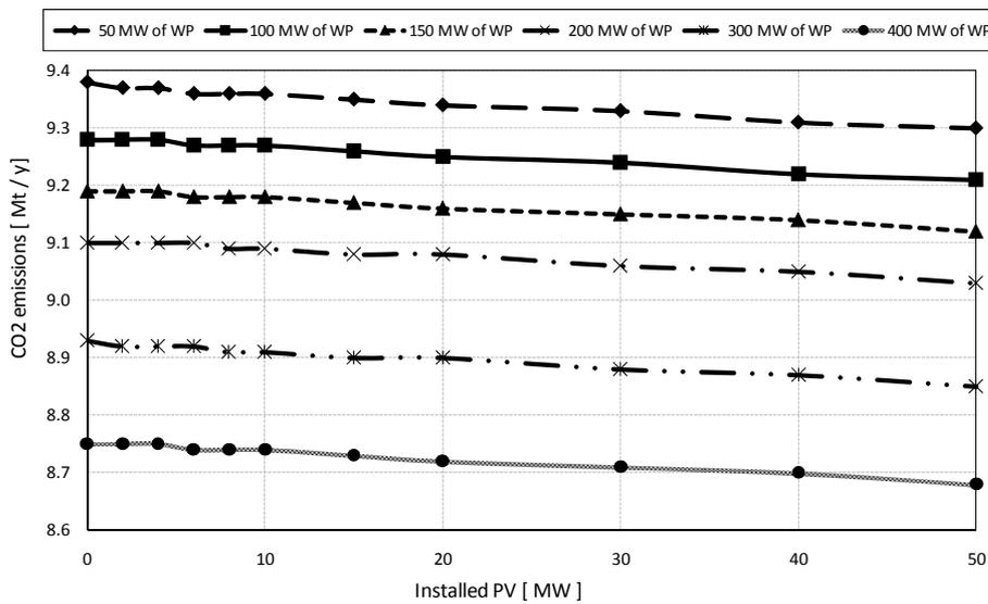
Fig. 1.: CO<sub>2</sub> emissions in the reference and closed energy system with the installed gas CHP plant and for different installed wind and PV capacity
