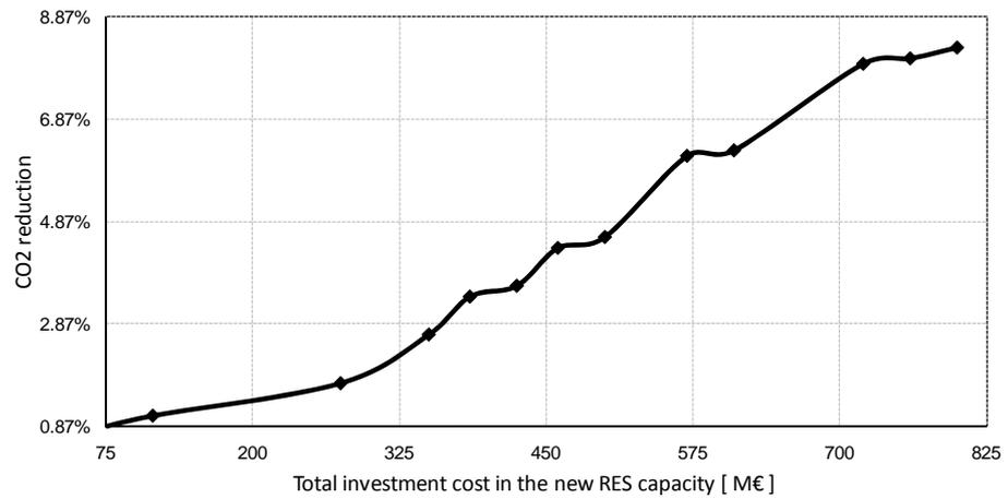
Fig. 2: Investment cost of the CO<sub>2</sub> reduction by wind and solar electricity
