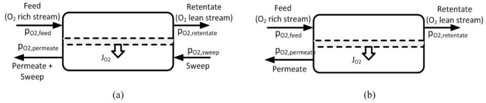
Figure 1: Process schematic of membrane operating method (a) with sweep gas and (b) without sweep gas
