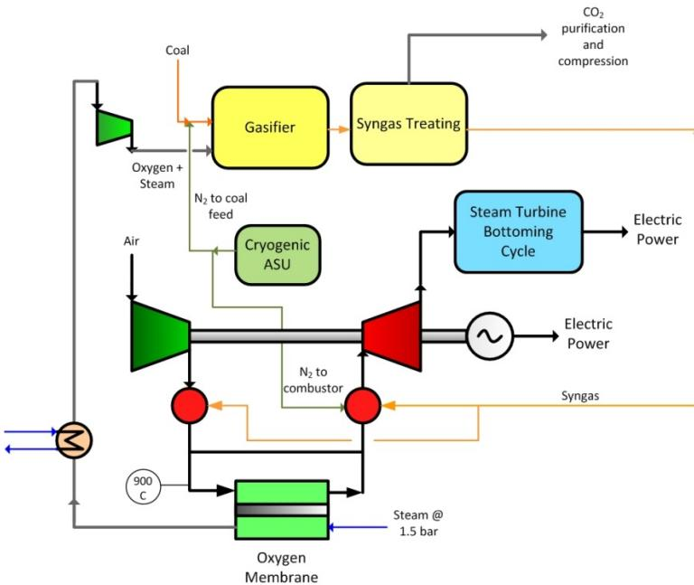
Figure 3: Process block diagram for OTM integrated IGCC plant with  $\text{CO}_2$  capture
