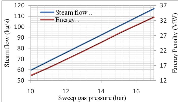
Figure 2: Sweep gas steam flows and associated energy penalty for extraction from bottoming cycle
