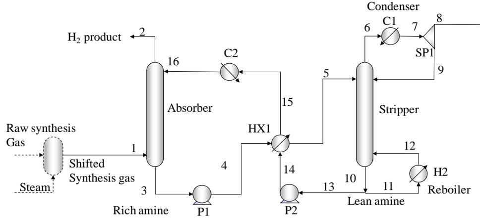
Figure 2: MEA absorption process (The conventional process)
