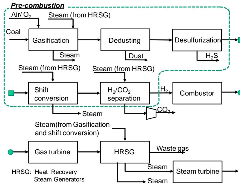
Figure 1: IGCC plant with pre-combustion CO<sub>2</sub> separation
