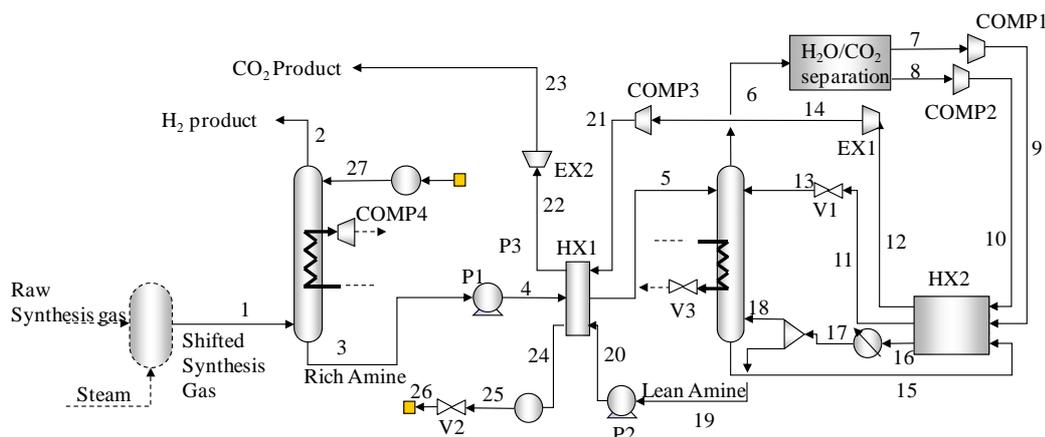
Figure 4: Absorption process based on self-heat recuperation thchnology
