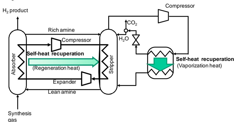
Figure 3: Conceptual design of exergy recuperative CO<sub>2</sub> gas separation process
