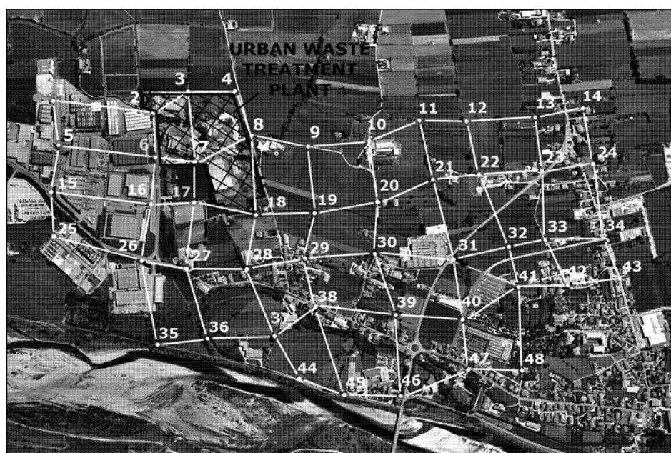
Figure 1: Municipal waste treatment plant localization in the assessment area with 48 measurement points and 33 measurement squares.
