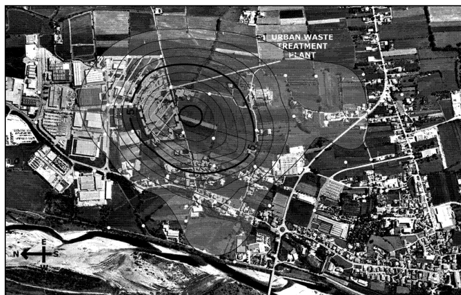
Figure 3: Isofrequency curves of biofilter odour
