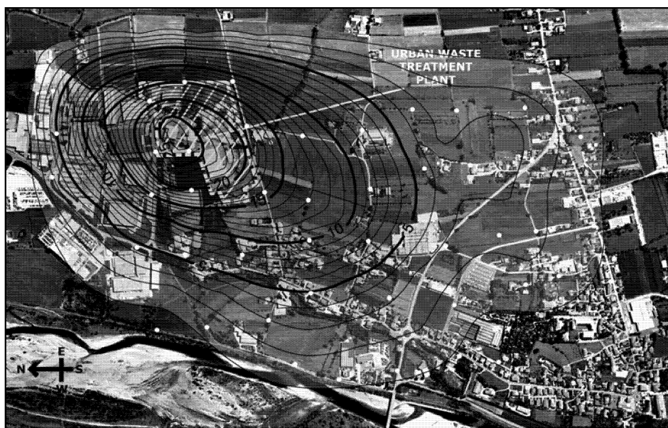
Figure 5: Isofrequency curves of total plant odour
