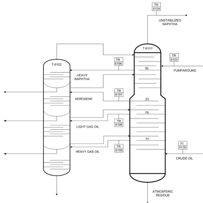
Figure 1: Crude distillation column with diesel fuel products
