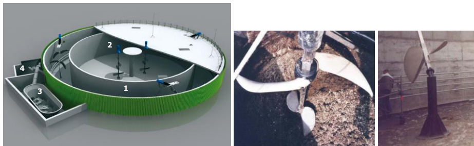
Figure 1: left: Basic principle of the biogas fermentation plant; 1: main fermenter, 2: post digestion tank, 3: feed system, 4: central pumping station. Mixing devices: center: type „Biobull“, right: „blade-agitator“.
