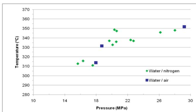
Figure 2: Experimental phase equilibria and modelling simulation for water - nitrogen and water - air binaries for different water composition.
