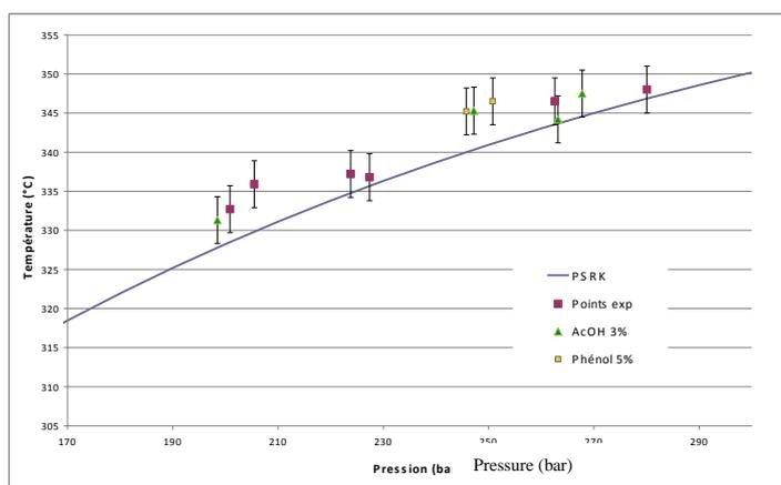
Figure 3: Experimental phase equilibria for water - nitrogen - waste ternary systems for different water composition.
