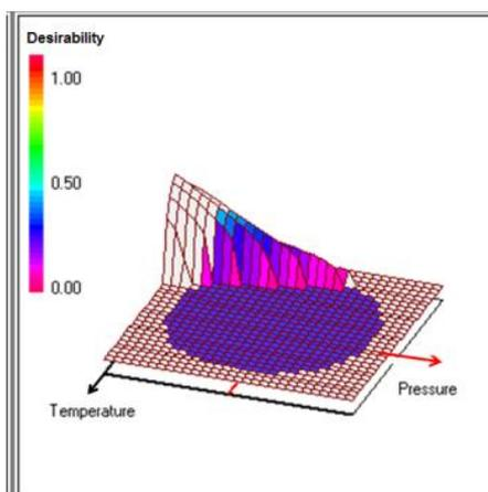
Figure 4: Evolution of the desirability function with temperature and pressure variation.
