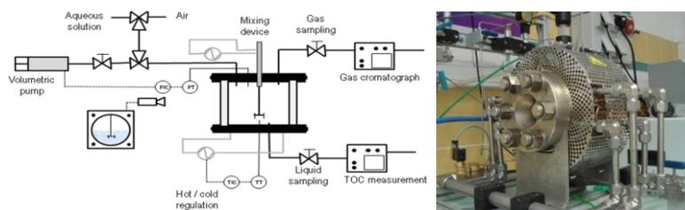
Figure 1: Experimental set-up for the measurement of phase equilibria
