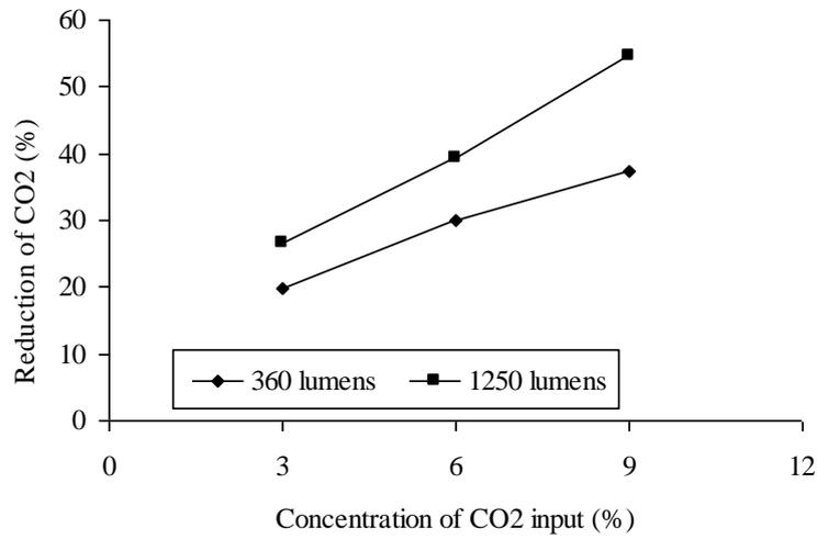
Figure 4. The effect of CO<sub>2</sub> input on CO<sub>2</sub> reduction
