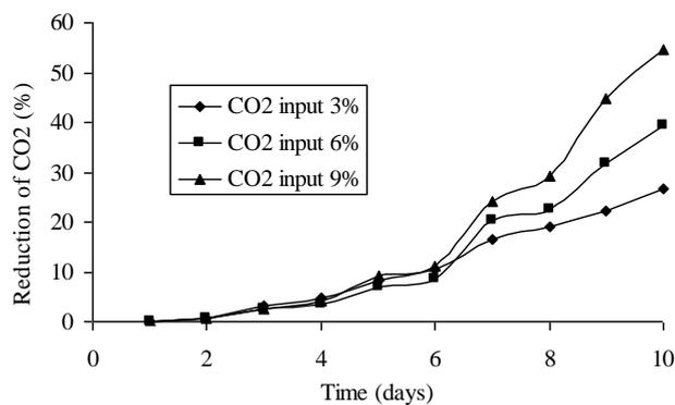
Figure 3: Reduction of CO<sub>2</sub> at various CO<sub>2</sub> input concentration with constant light intensity of 1250 lumen
