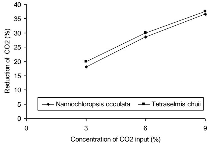
Figure 6: Comparison of CO<sub>2</sub> reduction by *Nannochloropsis oculata* and *Tetraselmis chuii* at light intensity 360 lumens
