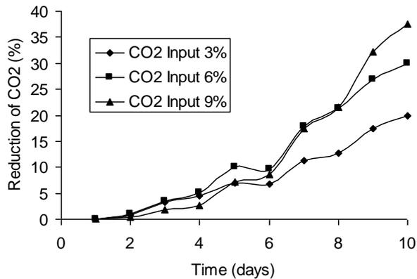
Figure 2.: Reduction of CO<sub>2</sub> at various CO<sub>2</sub> input concentration constant light intensity of 360 lumen
