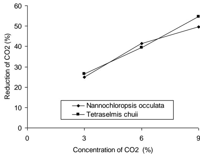
Figure 7 Comparison of CO<sub>2</sub> reduction by *Nannochloropsis oculata* and *Tetraselmis chuii* at light intensity 1250 lumens
