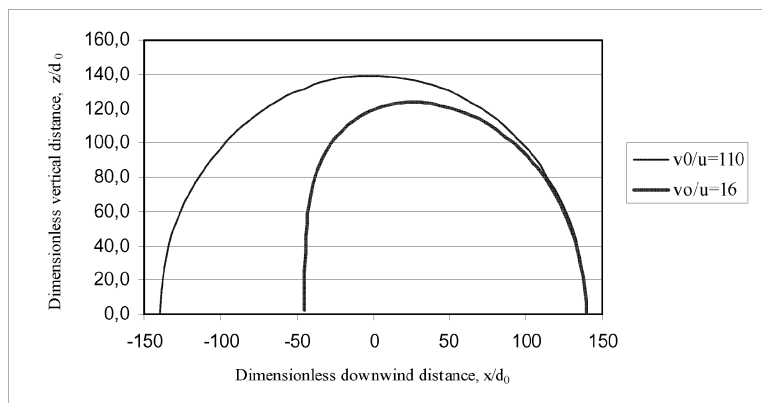
Fig. 2 Boundaries of the hazardous area, corresponding to LFL, for a n-heptane release, considering two different values of the velocity ratio v_0/u and the whole range of emerging angle 0 \leq \theta_0 \leq \pi .
