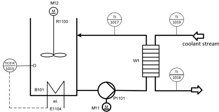
Figure 3: Piping and instrumentation diagram
