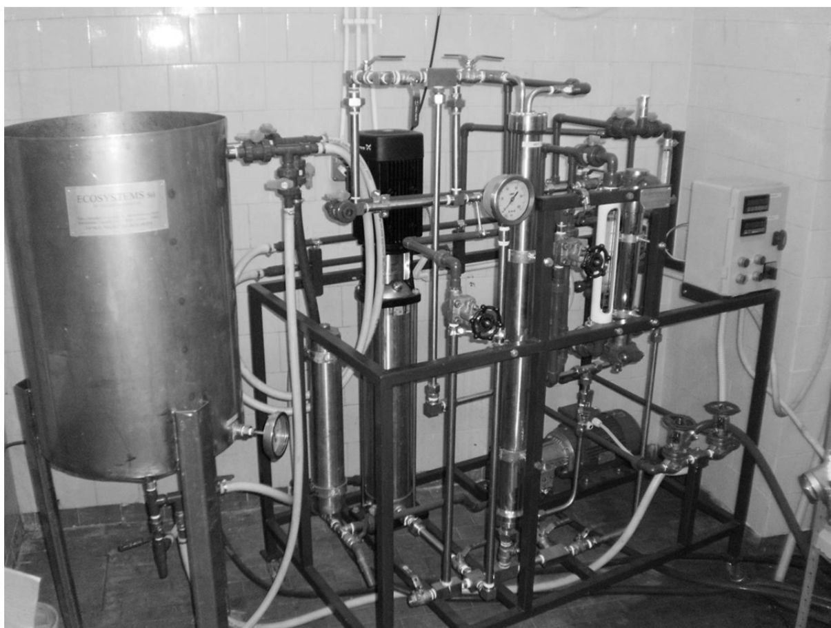
Figure 1 - Scheme and photograph of the pilot plant
