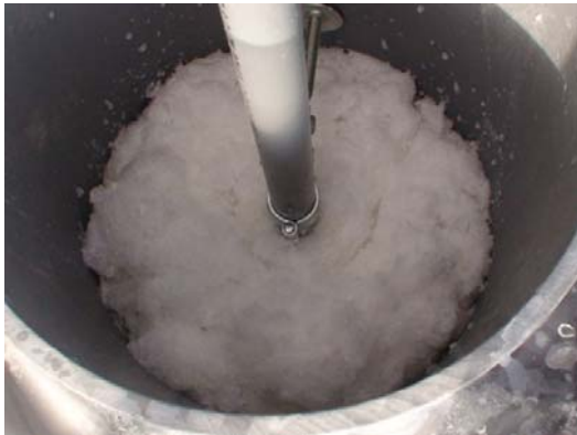
Figure 2: Foam at the upper part of reactor
