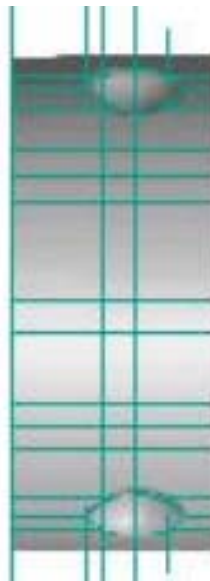
Figure 2: Mesh and center location used for the centerline CFD analysis on an enhancement character.
