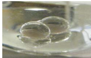
Fig.1 Two adjacent water in oil drops relying at the interface of two liquids
