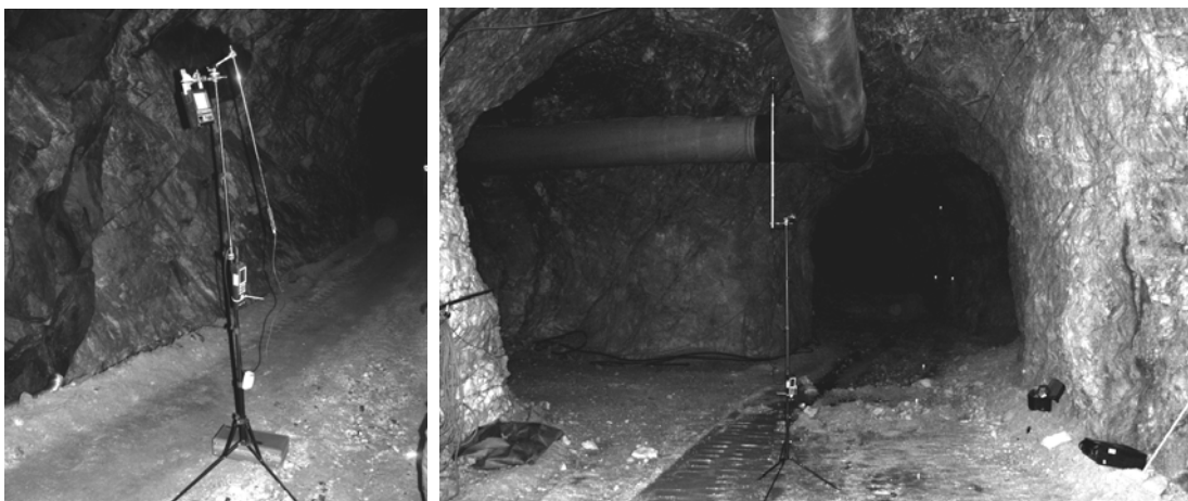
Figure 2, 3: measurement of the air flow in underground by means of an anemometer at node "N20"
