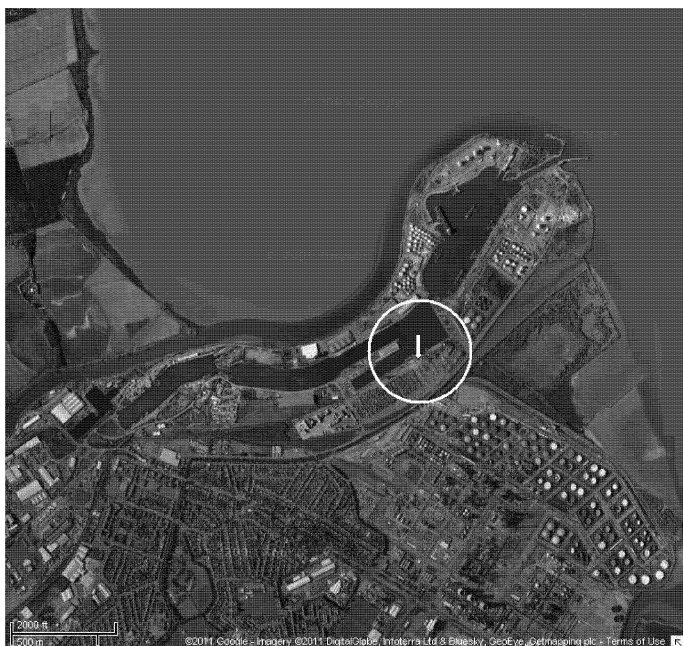
Fig. 9. Iso-risk curve for the release of DVB (the ray of the circle is equal to 220 m).
