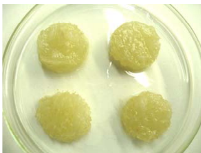
Fig. 1: loofa sponge- immobilized biomass of P.chrysosporium (LIBPC)
