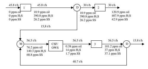
Figure 3 – Mass exchange network for regeneration and recycle with regeneration system.
