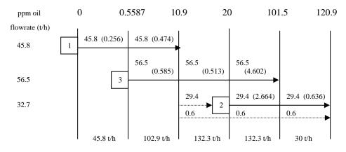
*Figure 2 – WSD for regeneration and recycle*
