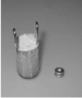
Left: Wire basket for traditional self-ignition tests (Grewer); right DSC crucible for the new method
