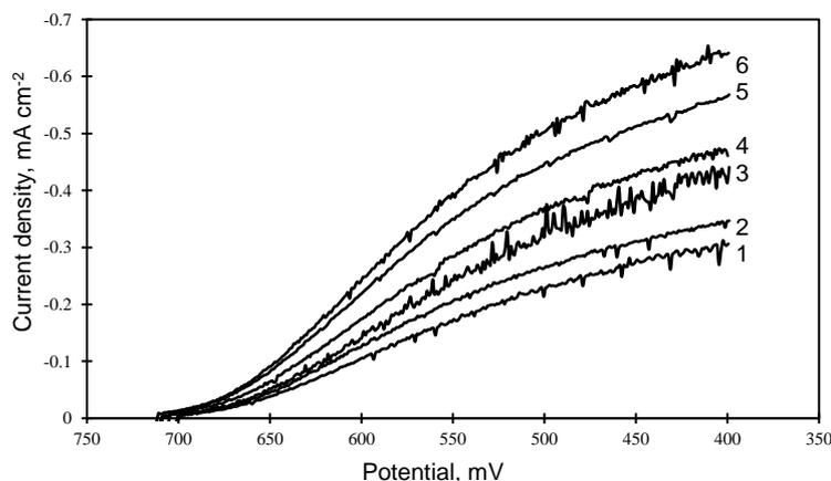
Figure 2: Polarization curves for the oxygen electroreduction by the electrode with laccase, adsorbed on CM CNT, which was pressed into the electrode with an amount: 1 – 0,37 mg; 2 – 0,46 mg; 3 – 0,48 mg; 4 – 0,73 mg; 5 – 0,86 mg; 6 – 0,94 mg. Potential sweep rate  $1 mV s^{-1}$
