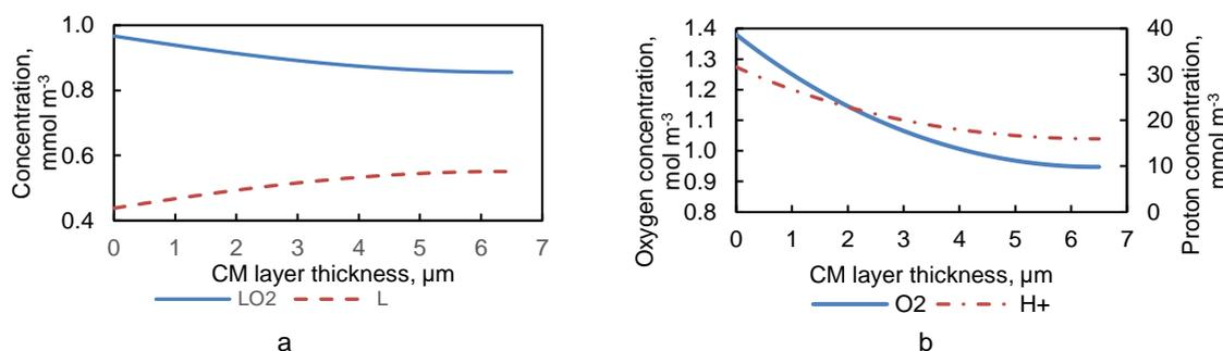
Figure 4: Calculated concentration distributions in the active layer: a) laccase and enzyme-substrate complex; b) oxygen and protons
