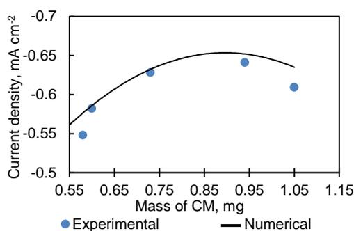
Figure 3: The experimental and the calculated volumes of the electrode activity on the loading of CM
