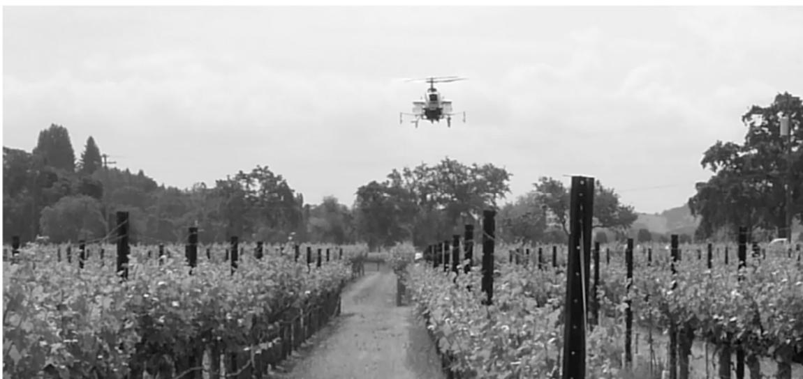
*Figure 2. Unmanned aerial vehicle (UAV) spray pass over vineyard as viewed by aircraft operator*
