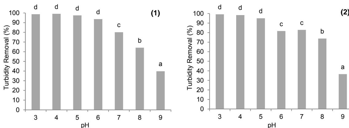
Figure 2: Turbidity removal in coagulation/flocculation tests using coagulants Tanfloc SG (1) and Tanfloc SH (2) the optimal dosage of 20 mg.L<sup>-1</sup> at different pH levels. Letters (a, b, c etc.) to identify different statistical graphs groups (Tukey test,  $p < 0.05$ )
