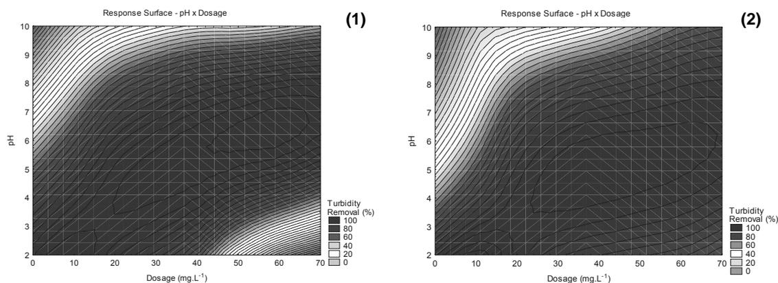
Figure 1: Response variable area for turbidity as a function of pH variation and dosage of coagulant (1) Tanfloc SG and (2) Tanfloc SH
