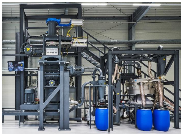
Figure 2. Used pilot plant, with pre-module (left) and product module (right)
