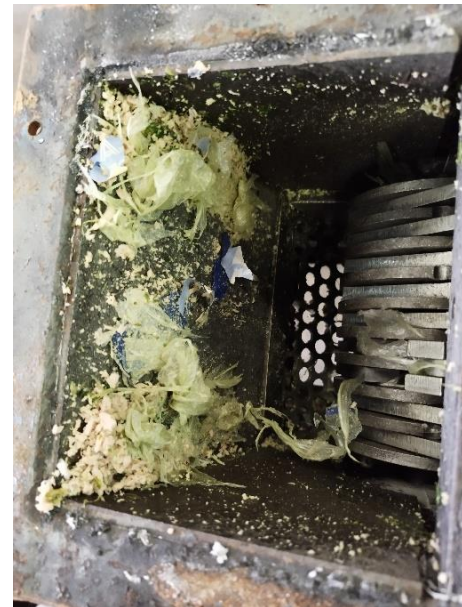
Figure 2. Test comminution in a hammer crusher.
