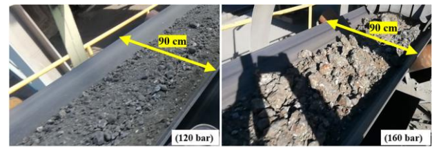
Figure 3. HPGR belt product in the operational pressures of 120 bar and 160 bar.
