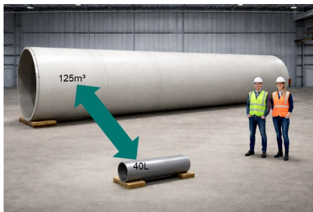
Figure 5. Comparison of system scale between a two-chamber tumbling ball mill ( \approx 125 \text{ m}^3 ) and a laboratory-scale agitated bead mill (Pamir 40 L), illustrating the large volume difference required to access comparable stressing regimes.
