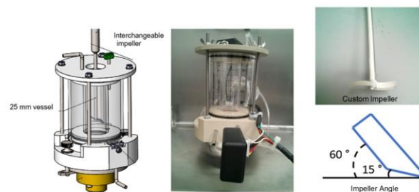
Figure 5. Experimental setup of the AFBD vessel. [14]
