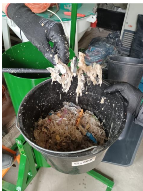
Figure 4. The skimmed materials which were floated on the surface of the suspension in the mixing tank.
