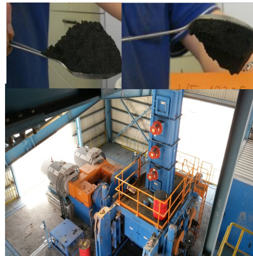
Figure 5. Stickiness of iron ore pellet feed and step feeder solution for HPGR
