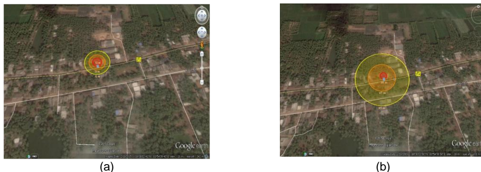
Figure 3. Simulated results (ALOHA) of thermal radiation with the damage distances of jet fire with release of natural gas (a) small leakage ( d_h = 0.05 \text{ m} ) and (b) full bore rupture ( d = 0.45 \text{ m} ) of pipeline.
