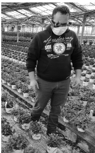
Figure 1. Operator wearing Smart Glasses combined with thermal imaging camera during on-field tests
